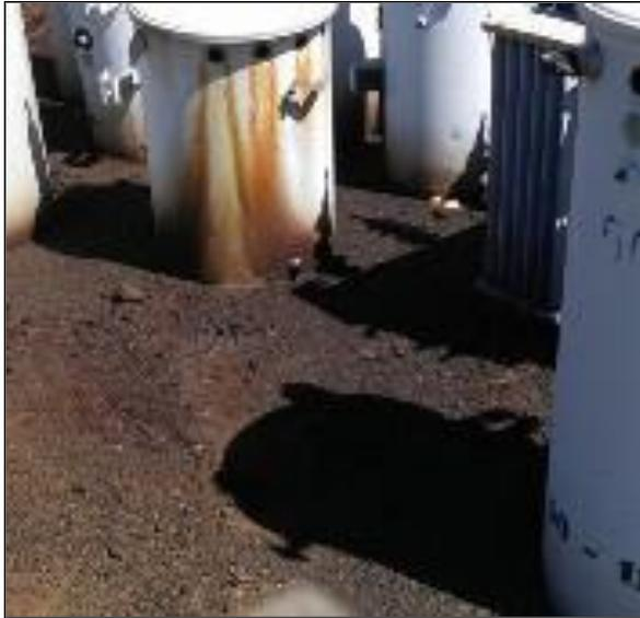
**Figure 2.15 Soil contamination associated with discarded distribution transformers - Sophia**
